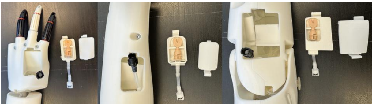
Figure 50 – Physical prototype of IV module with pre-ported and hidden (placeholder design) module variants. Dorsal veins IV site on left, cephalic veins IV site in middle, and cubital fossa IV site on the right.
